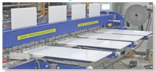
World class state-Of-the -art butt surface fusion technology for manufacturing of polypropylene pickling tank.
